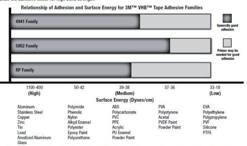
NOTES: There are a wide variety of formulations, surfaces finishes and surface treatments available on substrate materials which can affect adhesion. This chart is intended to provide only a rough estimate of the adhesion levels which can be expected on some common materials relative to a reference surface such as aluminum.
