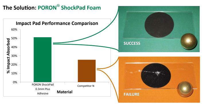
As you can see in the graph above, **PORON ShockPad Foam absorbs twice as much force as equivalent competitive material** in real-life drop conditions.
