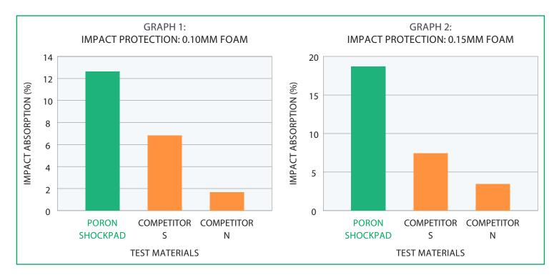
PORON ShockPad (0.10mm and 0.15mm) foam not only absorbs a significant amount of impact force, but displays excellent compression set resistance, is easy to process, and performs reliably over the life of the final product. To learn more, visit: Rogerscorp.com/ShockPad or contact your local sales representative.
